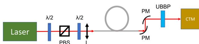
Fig. 3: Schematic of the experimental setup
