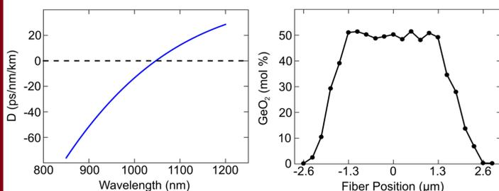
Fig. 2: Dispersion profile and germania concentration of the fiber
