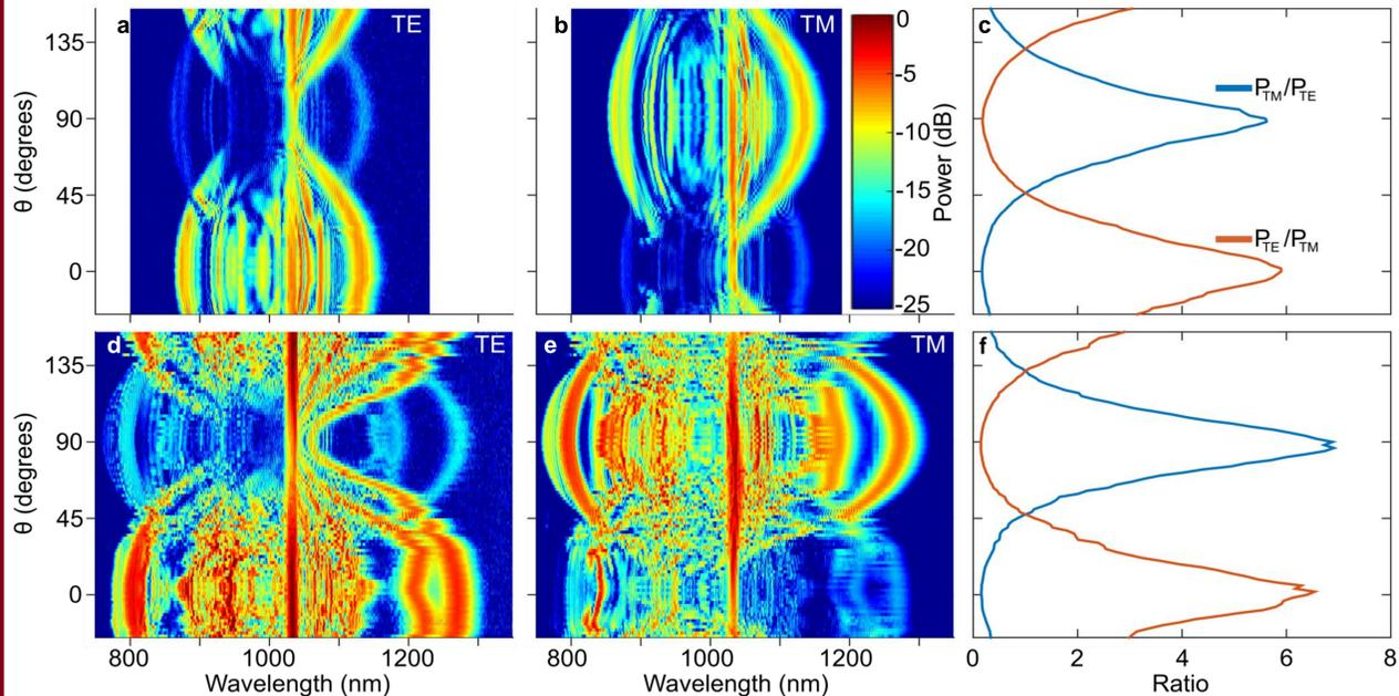
Fig. 4: Evolution of the SC spectrum at the output of the fiber as we rotate the input linear polarization at a fixed pulse energy of 0.3 nJ (a, b) and 1.1 nJ (d, e). c, f) Ratios of the TE and TM polarization components of the integrated spectra.
