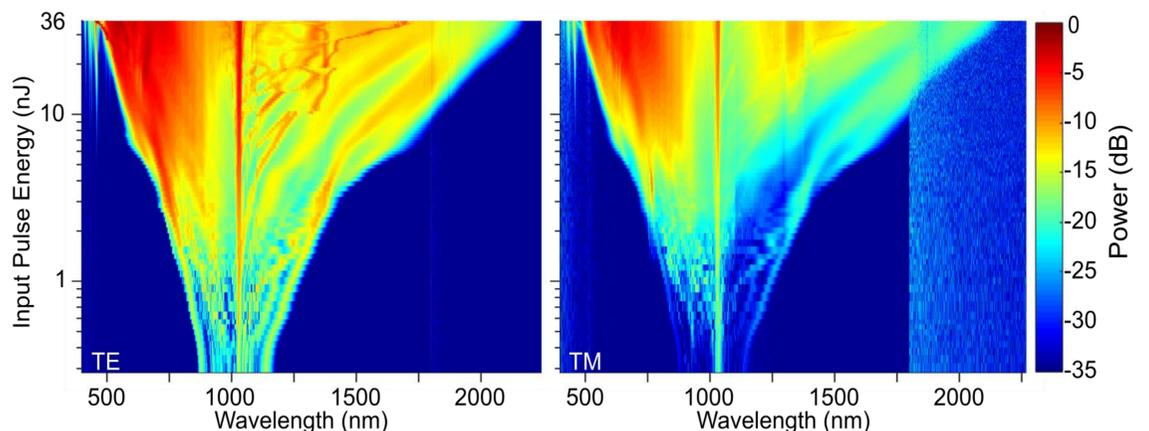
Fig. 5: Evolution of the spectrum (separated in its TE and TM components) as we increase the pulse energy launched in the fiber from 0.3 to 36 nJ. The input linear polarization is set along one of the principal axes of the fiber ( $\theta = 0^\circ$  in the Fig. 4)
