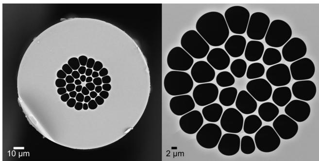
Fig. 1: Scanning electron microscope (SEM) image of the PCF
